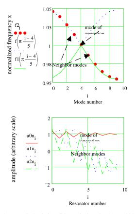
Figure 3: Numerical solution of the equivalent circuit ( $\gamma = .024$ ,  $\beta = 1, 1\%$  perturbation in the frequency of the first resonator) and dispersion relation for an infinite chain of resonators.
