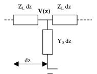
Figure 1: Equivalent circuit for the longitudinal dependence of the quadrupole modes a four vanes RFQ.
