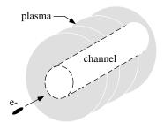
Figure 3: A hollow channel in a plasma can function as an accelerating structure.
