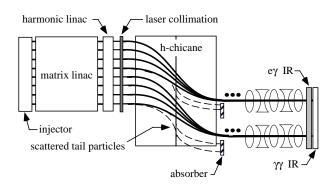
Figure 1: A new concept for a compact collider, as described by Zimmermann [2].
