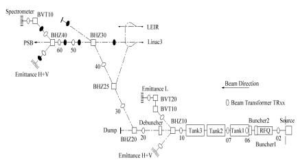
Figure 1: Schematic layout of Linac2 and its transfer lines.
