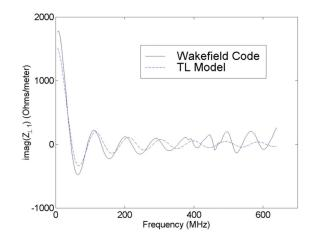
Figure 2 Dipole wake impedance
