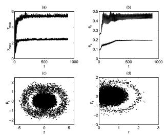
Figure 3: 6-D uniform distribution  $\mu_x = \mu_y = \mu_z = 1.5$ (c/a = 3,  $\eta_x = 0.53$ ,  $\eta_z = 0.39$ ) a) maximum x and z b) emittance growth c)  $z - p_z$  diagram at t = 900 (with 32,768 particles plotted) d)  $r - p_r$  diagram at t = 900for particles with the angular momentum  $|L_z| < 0.1$  (with 25,000 particles plotted).
