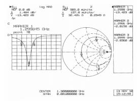
Figure 2: Reflection coefficient of gun cavity measured using HP8510C network analyzer.
