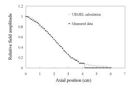
Figure 4: Longitudinal E-field profile on axis.
