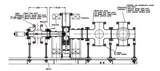
Figure 5: Layout of the L-band rf gun test stand.
