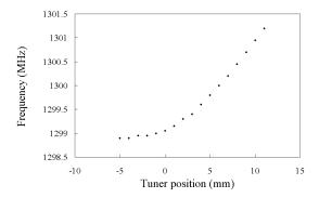
Figure 3: Measured resonant frequency dependence of tuner position.
