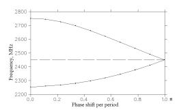
Figure 4: Dispersion curves for operating passband (experiment)
