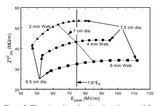
Figure 3: The points show the shunt impedances and the peak surface fields for 11 different cell diameters D and for 3 web thicknesses w, at the input energy ( $\beta$ =0.35).
