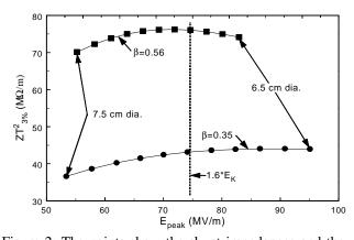
Figure 2: The points show the shunt impedances and the peak surface fields for 11 different cell diameters D, at the input ( $\beta$ =0.35) and output ( $\beta$ =0.56) energy. The web thickness w is 4 mm.
