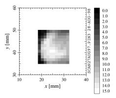
Figure 7. Map of the QE as a function of position on the surface of the second cathode the day after coating. Each pixel represents one QE measurement; the legend on the right indicates the QE values in percent.
