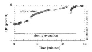
Figure 6. Comparison of the QE versus time before insertion into the gun and after rejuvenation for the second photo-cathode (UV power =  $10 \mu W$ , spot size = 5 to 10 mm).
