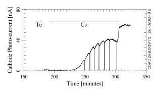
Figure 2. Photo-current as a function of time during the coating of the second photo-cathode. The times during which Te and Cs were being evaporated are indicated by the bars along the top. The downward spikes correspond to the UV light being blocked momentarily to check the background current.
