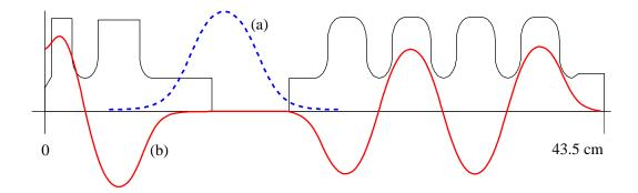
Fig. 1 Schematic of RF gun and booster showing (a) solenoidal magnetic field and (b) RF accelerating field.
