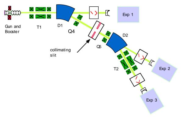
Fig.2 Schematic of the ELYSE accelerator showing the gun, booster, triplet magnets (T1, T2), dipoles (D1, D2), quadrupoles (Q4, Q5) and experimental areas (Exp 1, Exp 2, Exp 3).
