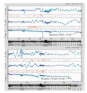
Figure 2: Two design beams have been achieved at the end of the linac: 8-GeV, 1.5-nC electron and 3.5 GeV, 0.5-nC positron beams.
