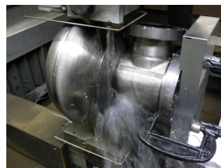
Figure 2: Removal of the end plate with an EDM.
