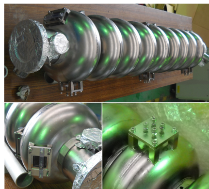
Figure 2: Photos of a 9-cell coupon cavity (upper), coupon holders and view ports near iris (lower left), a coupon holder near equator (lower right).
