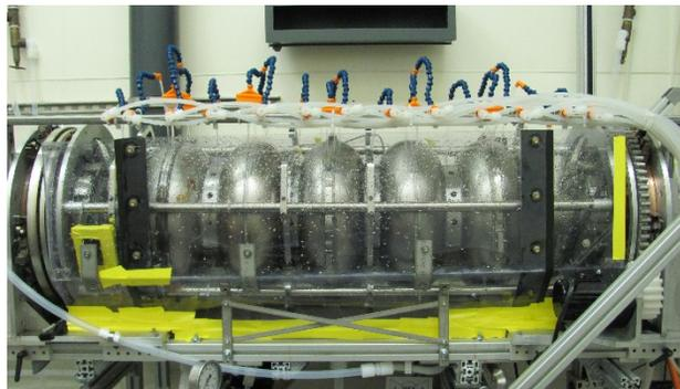
Figure 1: 650 MHz five-cell cavity EP with water cooling.
