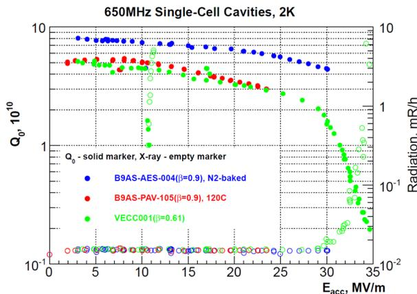
Figure 3: Single-cell 650 MHz cavity vertical test results.
