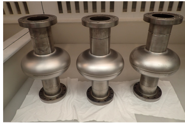
Figure 8: Three 1.3GHz Tesla shape single cell cavities.
