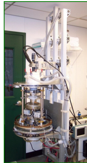
Figure 4: Faraday technology, Inc.'s Bipolar EP system [4].
