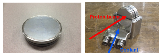
Figure 5: Prepared target (left) and target installed inside target holder.
