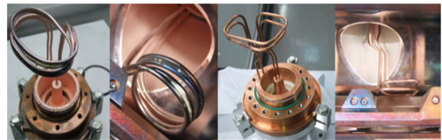
Figure 5: The former design of the coupler (left) and the upgraded coupler (right).
