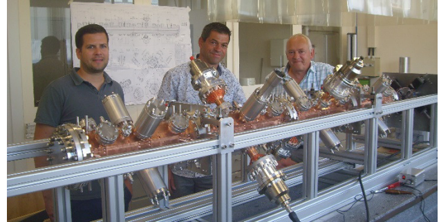
Figure 1: The RFQ assembled on the tuning bench.
