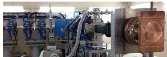
Figure 5: 8-MeV beam line and the target.
