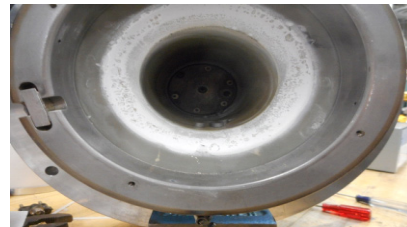
Figure 5: CsH film on the wall of the discharge chamber.
