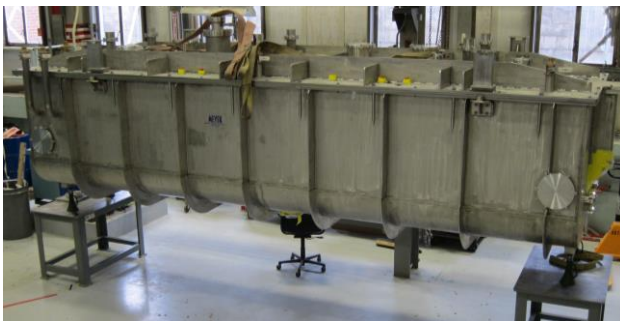
Figure 2: Picture of the cryomodule assembly prior to operating the 70 K coolant systems.
