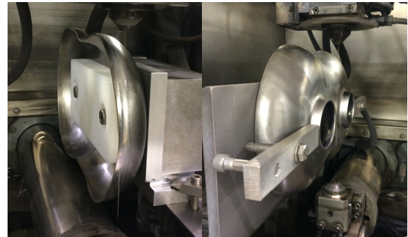
Figure 8: Wire EDM trimming of equator (left) and iris (right).
