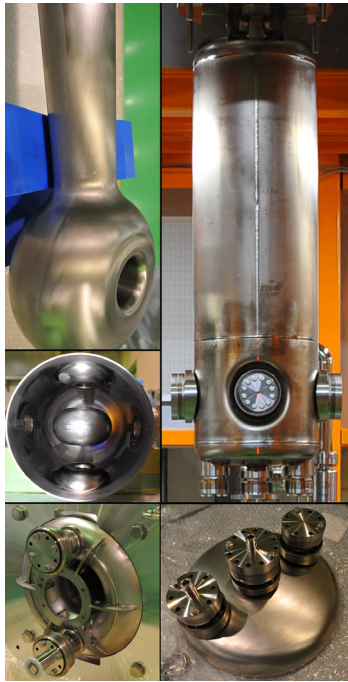
Figure 2: Photographs of the stem (upper left), inner view (middle left), top torus (lower left), bottom dome (lower right), and outward (upper right) of the SC-QWR prototype.
