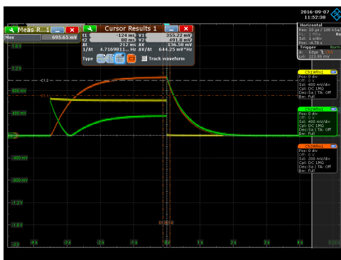
Figure 5: Forward, reflection, and transmission signal when the coupler position was at the inner limit (+10 mm). Green line indicates the reflection signal.
