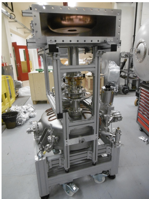
Figure 7: Power coupler with doorknob transition mounted on the test bench.
