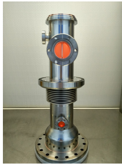
Figure 2: Warm External conductor.
