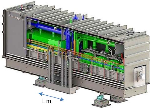
Figure 2:  $\beta=0.53$  pre-production CM modular bottom-up design. This CM incorporates 8  $\beta=0.53$  HWRs and 1 solenoid.
