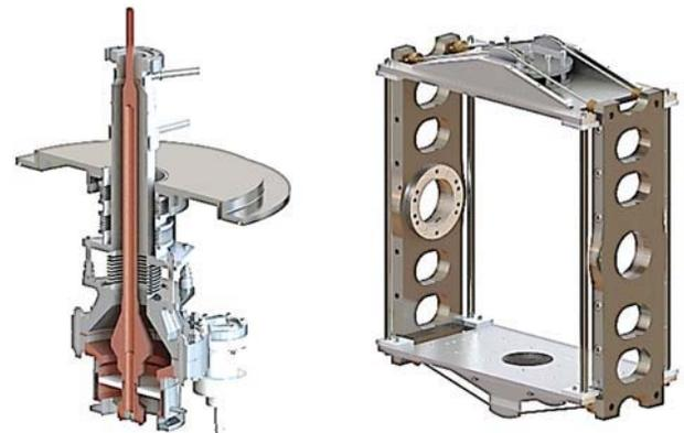
Figure 5: Half-wave power coupler assembly (left). Tuner mechanism by ANL (right).
