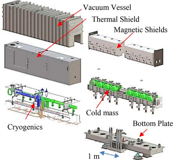
Figure 3: Sub-Systems of FRIB CM design. Supported off the bottom plate is the cold mass system, where the resonators are protected by local magnetic shielding (right). The cryogenic system attaches to the cold mass. All assemblies are encapsulated by the thermal shield and vacuum vessel (left).
