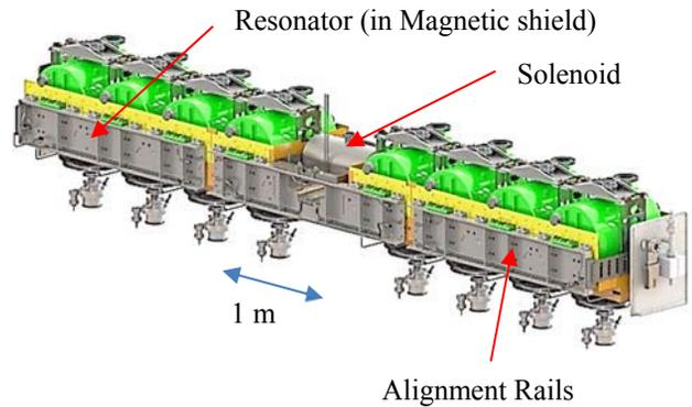
Figure 4: CM cold mass. Alignment rails support superconducting resonators and solenoid.
