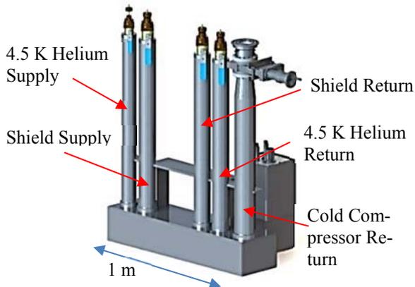
Figure 6: CM cryogenic bayonet box. The bayonet box connects to the distribution line by u-tube bayonets.
