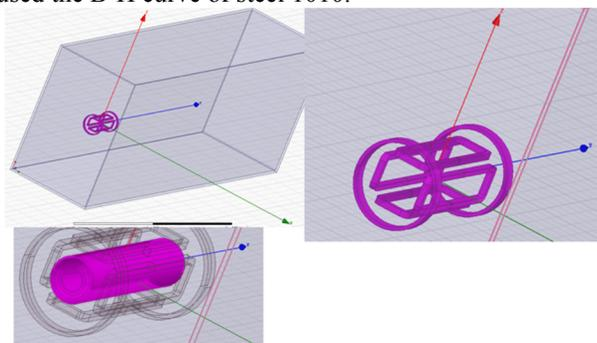
Figure 3: (Upper left) Cryostat with solenoid inside, (Upper right) Dipole coils and background coils, (Lower left) Nested solenoids.
