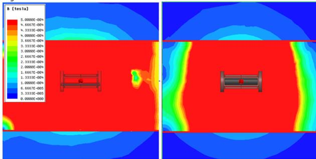
Figure 4: Top cross-section view of the cryomodule. (Left) Solenoid and bucking coil excited, (Right) Vertically bending dipole excited.
