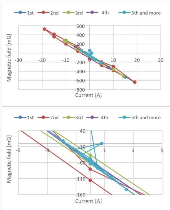
Figure 9: Magnetic field (y-direction: vertically bending dipole) vs. excited current. Lower is an enlarged view.
