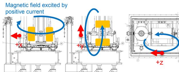
Figure 6: Measurement point and magnetic field direction excited by positive current: (Left) vertically bending dipole, (Middle) horizontally bending dipole, (Right) solenoid.
