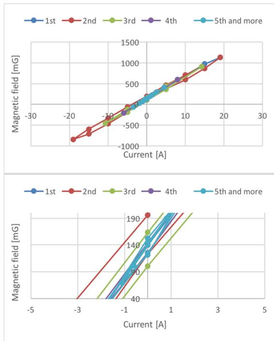
Figure 10: Magnetic field (z-direction: horizontally bending dipole) vs. excited current. Lower is an enlarged view.
