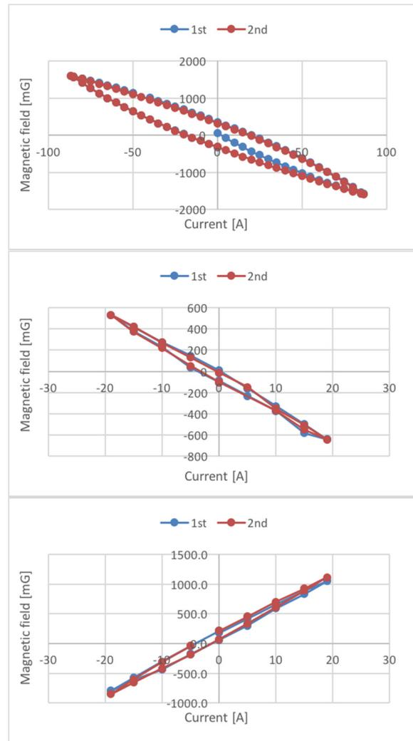
Figure 7: Magnetic field vs. excited current. (Upper) z-direction, (Middle) y-direction, (Bottom) x-direction.
