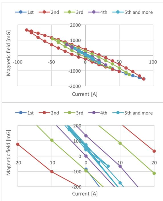
Figure 8: Magnetic field (z-direction: solenoid) vs. excited current. Lower is an enlarged view around the center of the upper plot.
