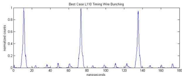
Figure 4: Time spectrum for bunched beam after the LINAC.
