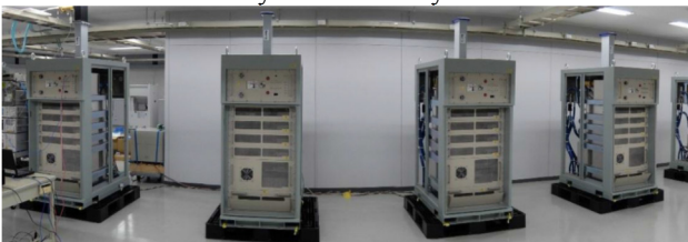
Figure 12: The first 1.3 GHz CW SSPAs for LCLS-II fabricated by R&K.
