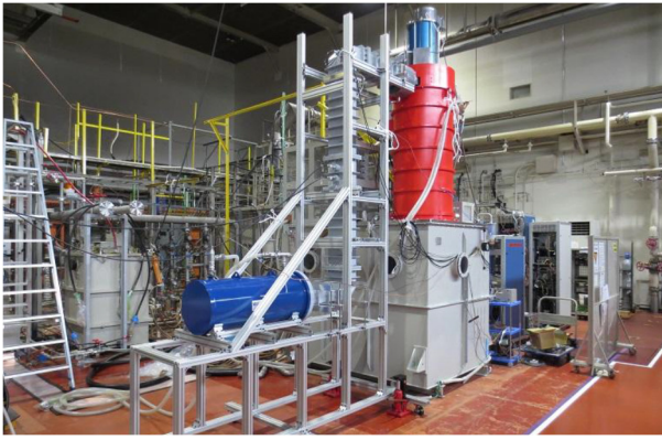
Figure 8: Prototype Toshiba 1 GHz MBK at Factory Acceptance Test (2016) [13].
