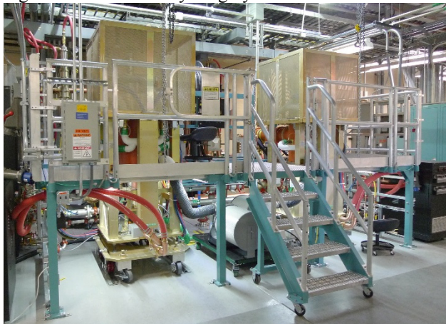
Figure 6: LANSCE 201 MHz, 3.4 MW RF power source with two Thales TH628L diacrodes.
