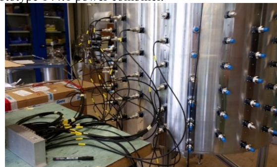
Figure 13: Prototype of a 144:1 cavity combiner during test set-up at CERN.
