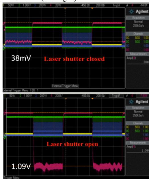
Figure 4: Faraday cup (1 MOhm) signal during the first beam test SRF 704 MHz SRF Gun. (Top: laser shutter closed dark current 38 nA. Bottom: laser shutter open photocurrent during RF pulse 1.09 uA).
