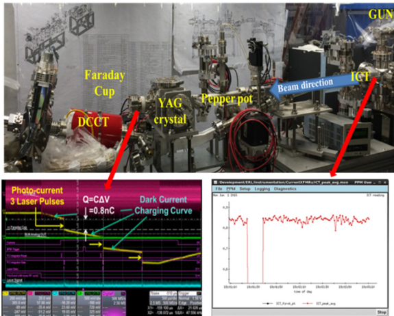
Figure 6: Straight beam line with beam diagnostics components (top). Dark current (slop) and photocurrent (spikes) measured one faraday cup (left bottom). Cross calibration charge measurements at ICT (right bottom).
