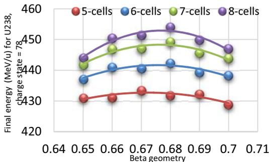
Figure 2b: Final energy  $^{238}\text{U}$ ,  $q=78$ , and  $E_i = 262 \text{ MeV/u}$  versus beta geometry utilizing FRIB energy upgrade 644 MHz linac. The purple represents the final energy for 8 cells cavity, the green for 7 cells cavity, the blue for 6 cells cavity, and the red for 5 cells cavity.
