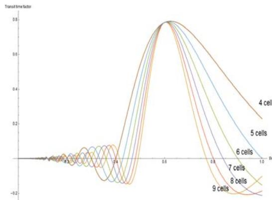
Figure 1: Transit Time Factor (TTF) vs. beta with varying number of cells (gaps) for elliptical cavities.
