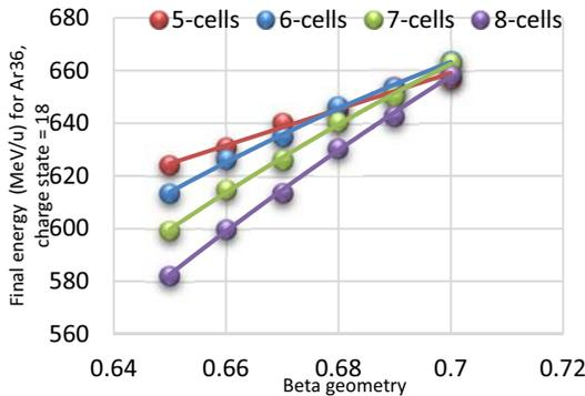
Figure 2a: Final energy gain for  $^{36}\text{Ar}$ ,  $q=18$ , and  $E_i = 401 \text{ MeV/u}$  versus beta geometry utilizing FRIB energy upgrade 644 MHz linac. The purple represents the final energy for 8 cells cavity, the green for 7 cells cavity, the blue for 6 cells cavity, and the red for 5 cells cavity.
