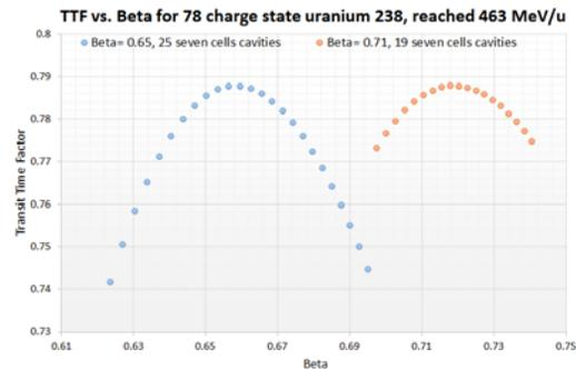
Figure 3: Transit time factor versus beta for  $^{238}\text{U}$ ,  $q=78$  reached 463 MeV/u at 644 MHz.
