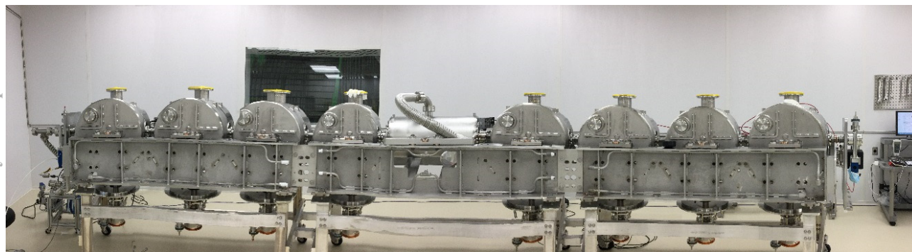
Figure 6: Assembled coldmass in cleanroom.
