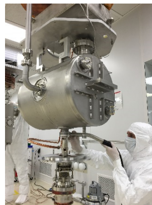
Figure 1: \beta = 0.53 cavity for vertical test on test insert with Fundamental mode Power Coupler (FPC).
