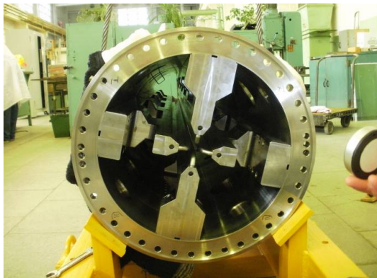
Figure 5: RFQ segment after first assembling and alignment.
