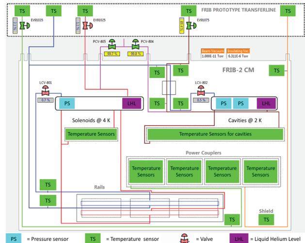
Figure 3: Diagram of the cooling system for cryomodule testing.
