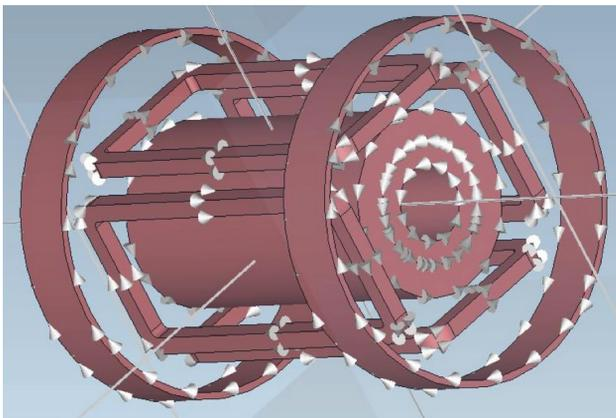
Figure 2: CST Studio model of the 50 cm solenoid package. Inner cylinder: main solenoid; intermediate rectangles: dipoles; outer rings: bucking coils. The diameter is 39 cm.
