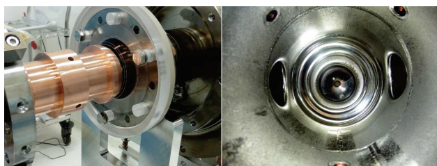
Figure 3: Left: Assembly and alignment of Petrov filter with acryl window. Right: Concentricity check by PEEK dummy cathode.
