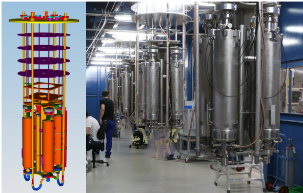
Figure 2: Inserts for the AMTF vertical tests. (Left) 3D schematic of an insert. (Right) inserts in the preparation area.
