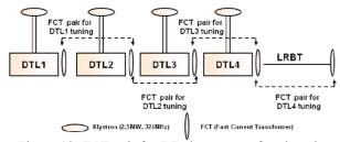
Figure 12: FCT pair for RF phase scan of each tank.
