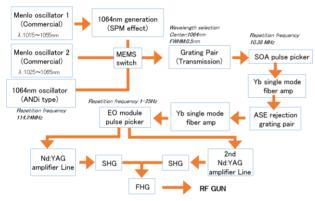
Figure 2: Layout of laser system.
