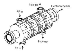
Figure 1: Technical design of the 4-cell fast corrector cavity with the 2 beamline flanges and the 4 feedthroughs for RF input and output loops/pickup.
