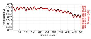
Figure 4: Maximum bunch transient amplitude in comparison to the charge measurement in the BC2 section. The black curve shows the maximum peak voltage and the red dashed line the charge readout for each bunch.
