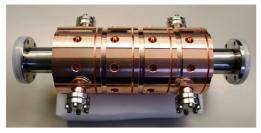
Figure 2: Assembled cavity after cell production, complete soldering and initial cleaning. The input and output loops are not connected.
