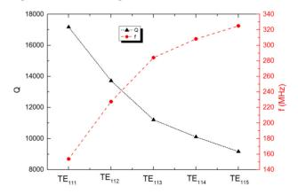
Figure 6: Resonated RF mode and Q values of calculated HOM-DTL. According to the TE<sub>11n</sub> order, the Q shows a downtrend and the frequency shows uptrend.
