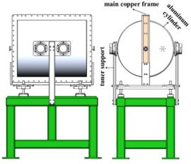
Figure 8: Assembly image of the HOM-DTL. The main frame is made from copper material, the other cavity parts (walls and the tuners) are being made from aluminium material.
