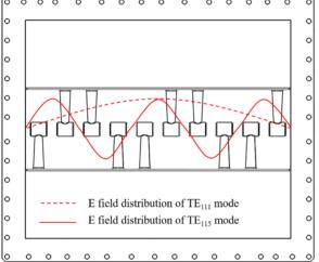
Figure 4: RF property of TE<sub>115</sub> mode (solid line) in the HOM-DTL. Dot line shows a RF property in IH-DTLs.
