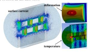
Figure 7: Images of surface current (left part) and multiphysics analysis. The intensity increases as the color changes from blue to yellow and to red.
