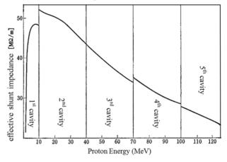
Figure 2: The shunt impedance changing of the Alvarez type DTLs.
