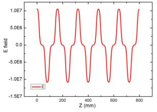
Content from this work may Figure 5: A flat e field distribution of TE<sub>115</sub> mode in the HOM-DTL.
