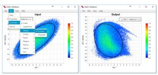
Figure 3: Longitudinal phase space input/output distribution of a LORASR-simulation, plotted with color-coded density. Beside the standard rainbow-colormap, perceptuallyuniform colormaps will be implemented to ensure printability in color and grayscale as well as for being viewed by persons with a color vision deficiency, too.
