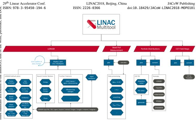
Figure 2: Feature diagram of the LINAC-Multitool giving an overview of the so far planned subprograms.
