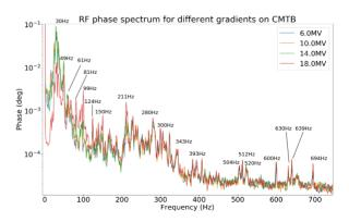
Figure 4: Microphonic noise recorded on the probe signal of cavity 1 at different accelerating voltages.  $Q_L = 5 \cdot 10^7$ .
