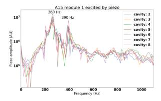
Figure 3: Transfer function between excitation produced by the fast tuner and piezo sensor.
