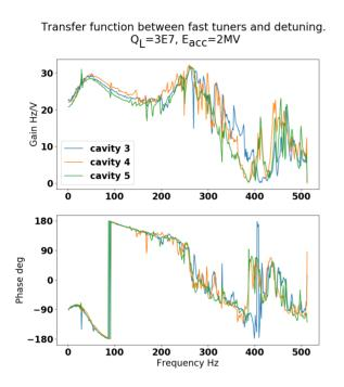
Figure 5: Mechanical transfer function between piezoelectric actuators of cavity 3,4,5 XM-3 and probe signals. The Y axis is the amount of detuning produced by a sinusoidal excitation from the piezoelectric actuators.
