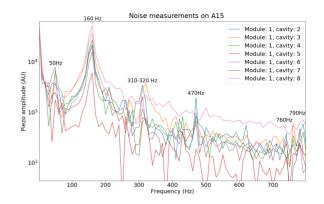
Figure 2: Microphonics recorded at European XFEL RF station A15 cryomodule 1 with piezoelectric sensor. Cavity 1 is not shown.
