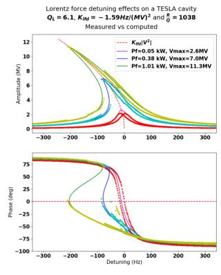
Figure 1: Resonance scan of a TESLA-like superconducting cavity at different values of the forward power using piezoelectric actuators. Computed (lines) vs. measured (points) values are shown. Tests were taken on cavity 2 of XM-3 module.
