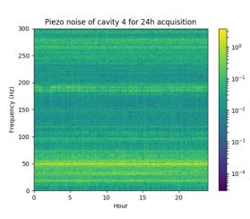
Figure 6: Noise spectrogram taken during a 24h data recording. The signal is recorded from a piezoelectric sensor.
