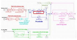
Figure 3: The closed-loop control block diagram of digital controller DPC of Swiss light source.
