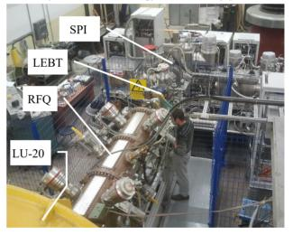
Figure 4: New fore-injector for LU-20.
