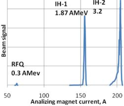
Figure 3: Measurements of the beam energy at the exit of HILac in three steps of acceleration combined in one picture: only RFO acceleration, RFO+IH1, and full linac energy.
