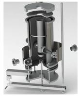
Figure 7: General view of 162 MHz QWR design model.
