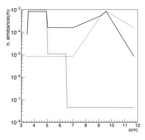
Figure 3: Emittance evolution of the simulation. The horizontal axis shows the distance from the cathode, and the vertical axis shows the normalized emittance in m.  $\varepsilon_x$ ,  $\varepsilon_y$ , and  $\varepsilon_z$  are drawn with solid line, dashed line, and dotted line, respectively.
