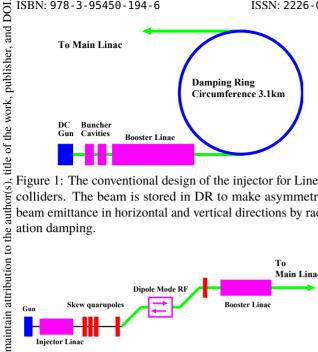
Figure 1: The conventional design of the injector for Linear colliders. The beam is stored in DR to make asymmetric beam emittance in horizontal and vertical directions by radiation damping.
