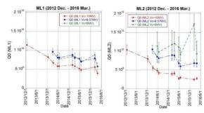
Figure 2: Measurement of the Q-values of 6, 8.57 and 10 MV cavity voltage during long-term beam operation from 2012 to 2016 including high power test of Main linac 1(left) and 2 (right).
