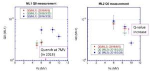
Figure 7: Q-value measurement results of ML1(left) and ML2(right). Horizontal (vertical) axes show the cavity voltage (Vc) and unloaded-Q values of both cavities.
