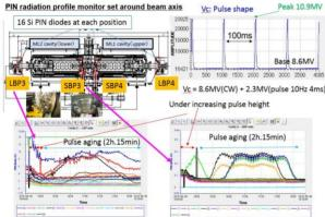
Figure 6: Pulse processing condition for ML2 cavity at 9<sup>th</sup> phase. Lower figures shows the trend of the PIN diode signals set on the both ends of ML2 cavity under the pulse processing as shown in the upper left figure of this figure.
