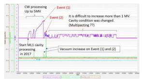
Figure 3: ML1 cavity processing trend on 8<sup>th</sup>.Mar.2017 before beam operation. Purple (pink) line shows the cavity voltage in ML1 (ML2). Green (line blue) line shows the vacuum inside the cavity of ML1 (ML2). Green (light blue) line shows the vacuum inside the cavity of ML1 (ML2). Brown (Gold) line shows the vacuum in warm side of the input coupler of ML1 (ML2).
