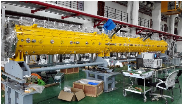
Figure 3: RF low-power measurement of DTL cavity.
