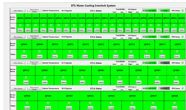
Figure 5: DTL water cooling interlock system.
