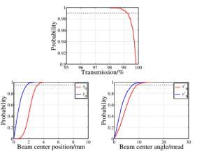
Figure 7: Probability of the transmission rate of the DTL (top), beam center position (bottom-left), beam center angle (bottom-right) at the end of the DTL after changing the input beam.
