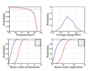
Figure 6: Probability of the transmission rate (top-left), the average energy (top-right), beam center position (bottom-left), beam center angle (bottom-right) at the end of the DTL.
