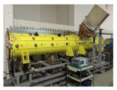
Figure 1: CPHS DTL cavity.
