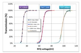
Figure 7: Transmission of the 3 references particles.
