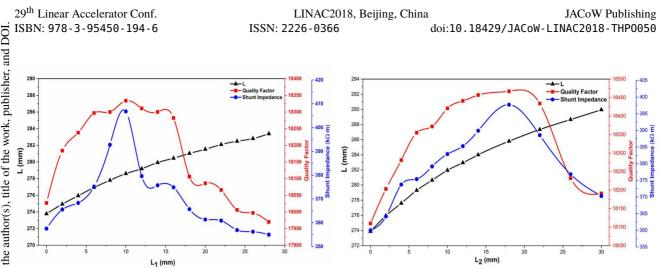
Figure 5: The variation of the lateral dimension (L), quality factor and shunt impedance of the bent-vane RFQ as the functions of the parameters of the cross-section profile (Only presenting two parameters).
