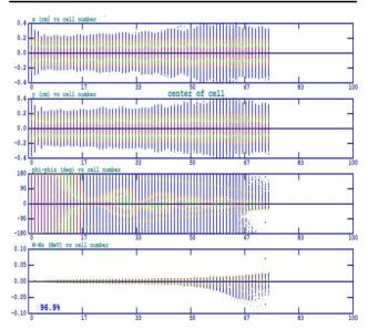
Figure 1: Beam dynamics simulation of the bent-vane RFQ (RFQGen).
