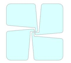
Figure 4: The slice model of the bent-vane RFQ.
