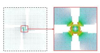
Figure 3: The electric field distribution of the bent-vane RFQ.
